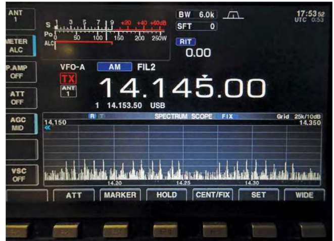
Figure 2 — The Icom IC-7700 receiver power line noise S-8 reading, and spectrum display, using the AM detector, with a 6 kHz bandwidth.
