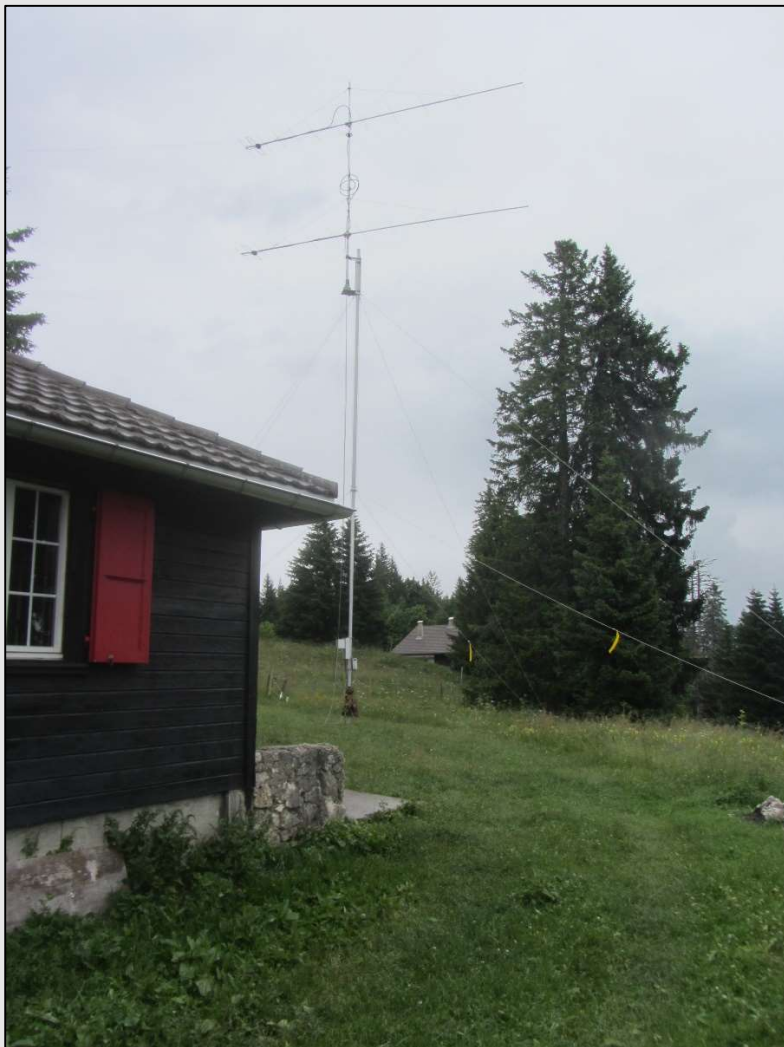
HB9N – JN37KB (NE) - 2x13ele Yagi, 145 MHz
