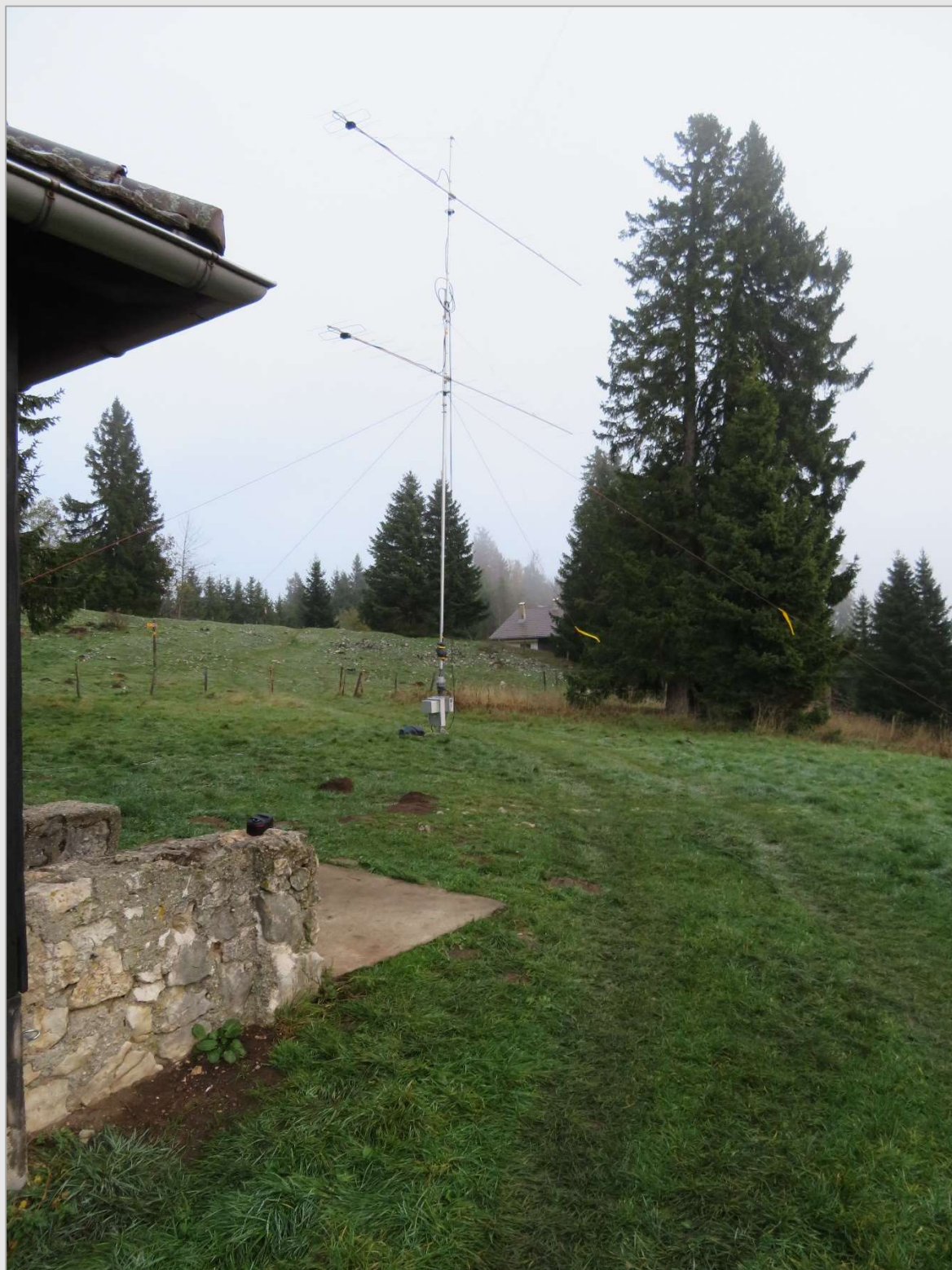
HB9N, QTH JN37KB (NE) 2x 13 element yagi for 144 MHz
