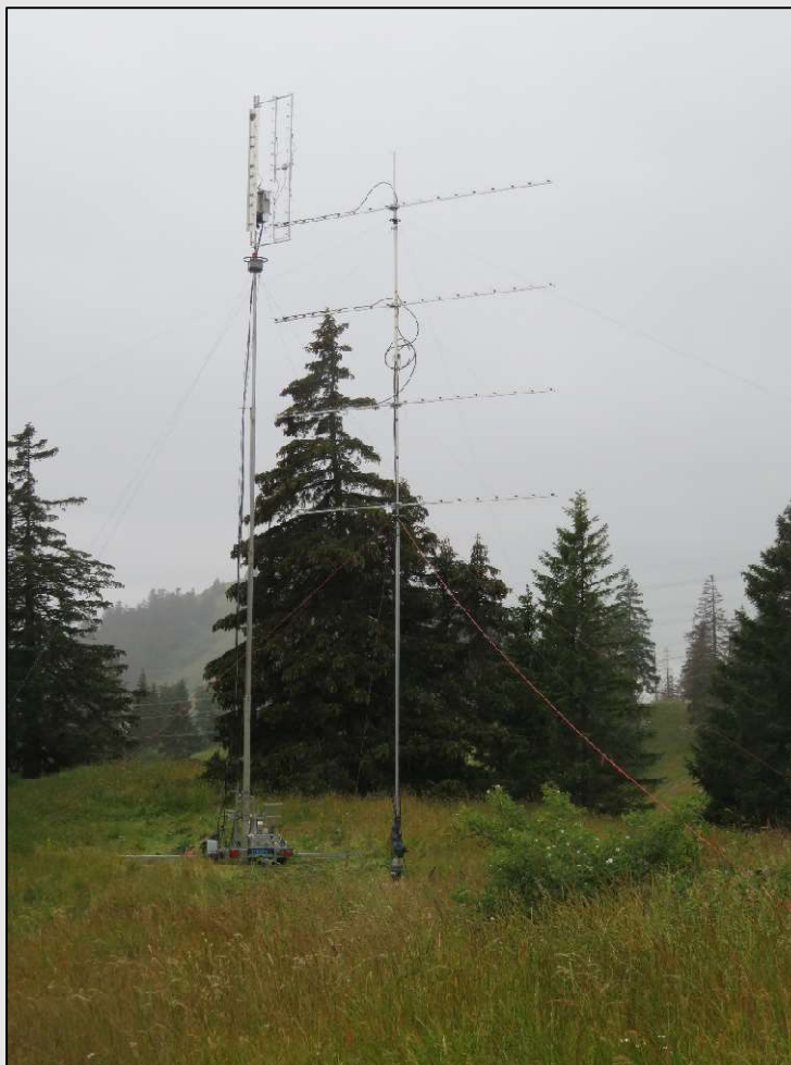
HB9N – QTH JN37KB (NE) – 4x20ele for 432 MHz, Panel-Antenna for 1296MHz
